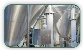
FERMENTATION TANKS, CYLINDRICAL-CONICAL TANKS (CCTS), AND BEER DRAW-OFF LINE
